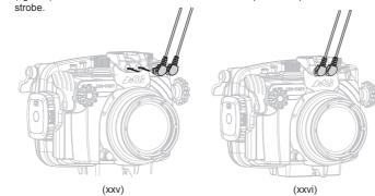
c. The flash trigger signals (electrical signals) will be transferred from the camera Hot Shoe to the Multi-control Device through the Hot Shoe Connector (included in the package). The Optical Flash Trigger in the Multi-control Device will convert the electrical flash triggering signals into optical signals and then will deliver them to the Fiber Optic Cable. The Fiber Optic Cable (not included in package) picks up the optical signals and delivers them to the external strobe
